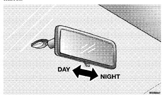
Annoying headlight glare can be reduced by moving the small control under the mirror to the night position (toward rear of truck). The mirror should be adjusted while set in the day position (toward windshield).
